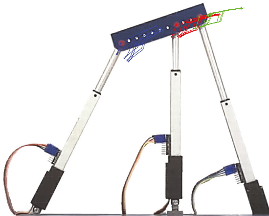
Figure 11. Trajectories of the first (blue), second (red) and third (green) manipulator platform joint during the dynamic experiment. The trajectories were recorded by a camera with 30 fps and the joints' positions were analysed using image processing.
