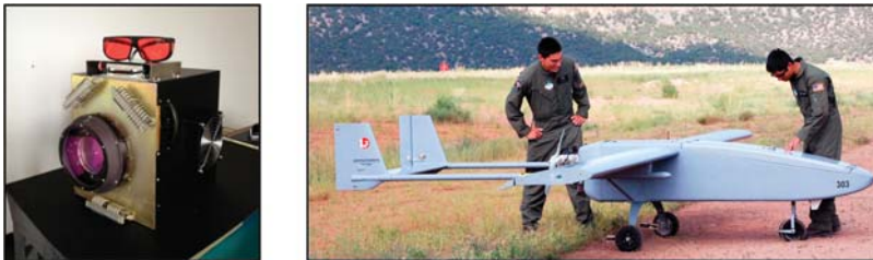
Figure 4. NASA Mini-ATM (Airborne Topographic Mapper) and its designated host aircraft, the Viking 300 micro-UAV.
