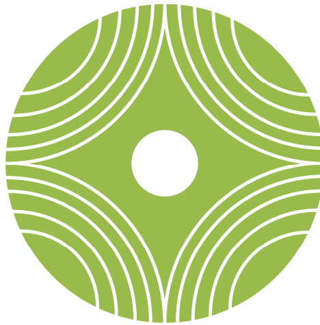
Figure 37. SynRM with axially laminated rotor [23].
