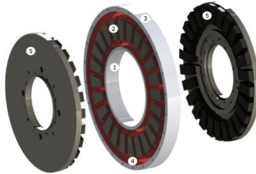
Figure 4. Yokeless and Segmented Armature Axial Flux Permanent Magnet Synchronous Machine: (1) Thermal end-winding interconnection ring (2) Concentrated winding tooth coil (3) Aluminium housing (4) Epoxy impregnation (5) Permanent magnet rotor.
