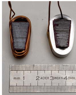
Figure 7. Prototype tooth coils. Left: enamelled copper wire tooth coil, Right: anodised aluminium foil tooth coil.
