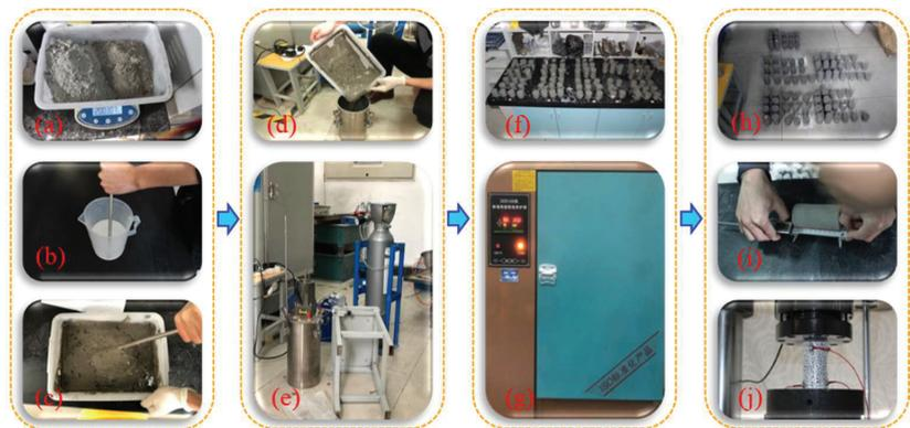
**Figure 3.** The process of CMFB specimen preparation and the mechanical tests.
