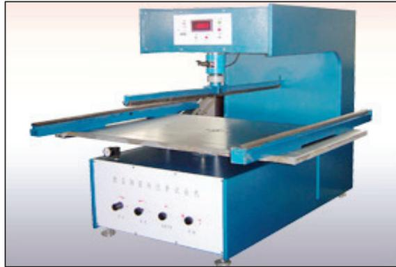
Figure 5. TZS-type digital flexural testing machine.
