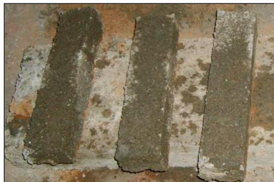
Figure 6. The flexural strength specimens.
