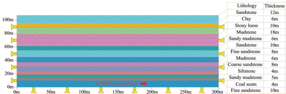
Figure 5. Numerical model to simulate the HWCZ of the CEPB mining method.
