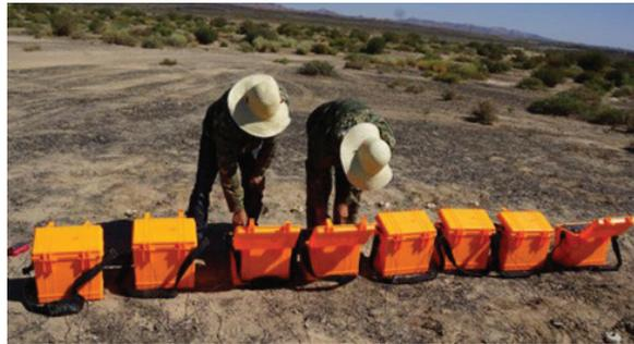
Figure 4. The receivers of the DEM system.
