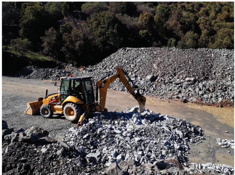
**Figure 10.** Secondary breaking of fragments.
