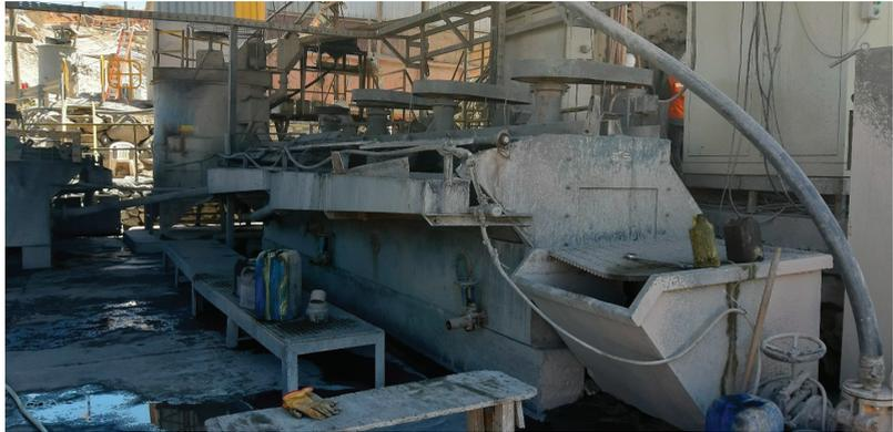
Figure 18. Flotation cells.
