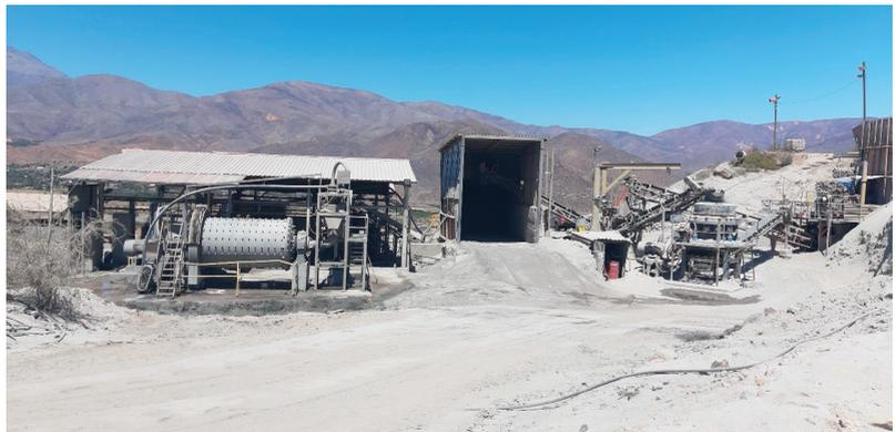
**Figure 17.** Crusher and mill at the plant.
