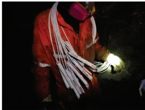
Figure 8. Explosives handling (incorrect and dangerous).
