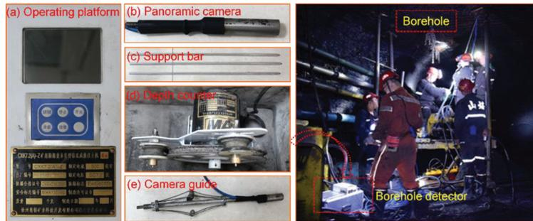
**Figure 12.** Field measurement of borehole television logging for determining the HWCZFZ. (a) The operating platform for borehole television logging. (b) The panoramic camera. (c) The support bar to transport the camera to the detection position. (d) The depth counter to measure the distance from the starting point of the drillhole to the detection position. (e) The camera guide to make it easy for the camera to pass through.
