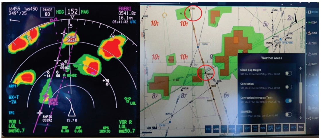
Figure 1. (Left hand): Photograph of the on-board radar display of a Lufthansa flight with heading 152 degree near way-point EGEBI (China) towards waypoint PADNO. The NCS-A information (right hand) provided in the EFB tablet computer in the cockpit supports situational awareness, e.g., that the passage of the southeast way-point PADNO could be possible and that there is likely no strong convection behind it (in the South, the lower part of the map).
