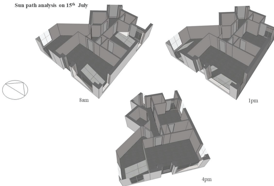
Figure 21. 8th Floor Base model in DesignBuilder: internal 3D layout with sun path analysis at different times on 15th July.
