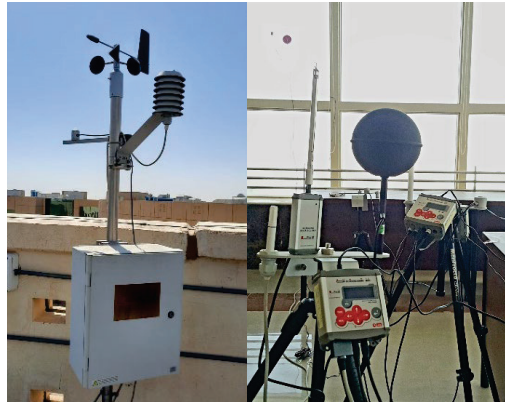
Figure 6. Data loggers for indoor and outdoor environments (LSI-R-Log and LSI-E-Log Weather Station).
