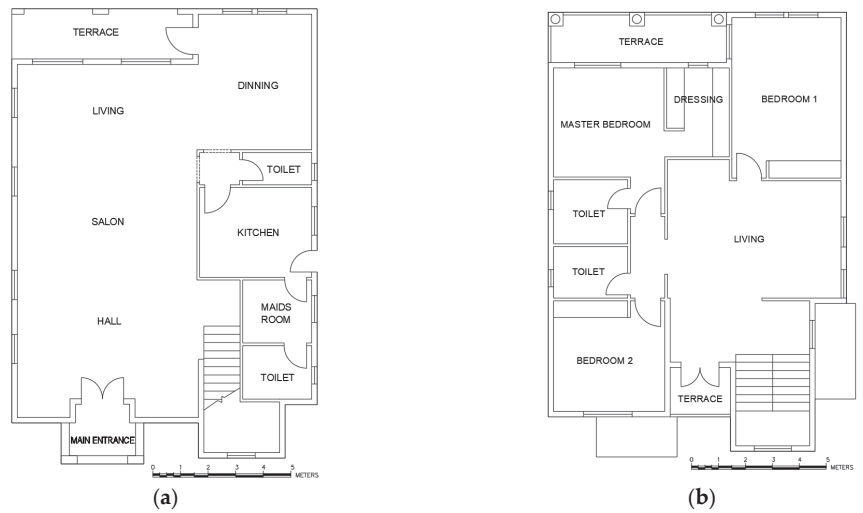
Figure 6. Representative dwelling model for villa model B: (a) ground floor (b) first floor.
