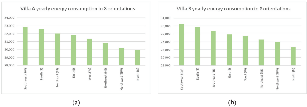
Figure 10. Yearly energy consumption in eight orientations for (a) villa model A and (b) Villa model B.
