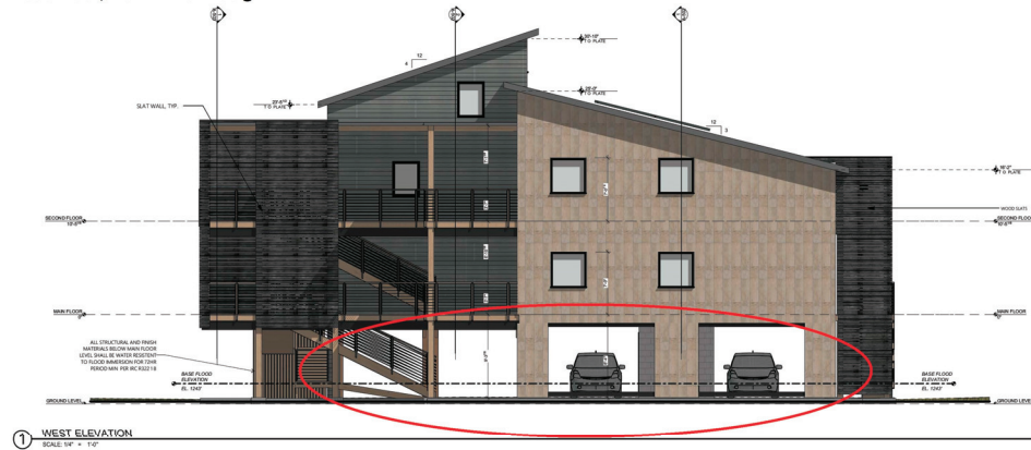
Figure 2. Everly House design from May 2022, building is ground-supported and 2 stories above ground level (circled in red) (top) to December 2022, building is raised on piles (circled in red) and three stories above ground level (bottom).
