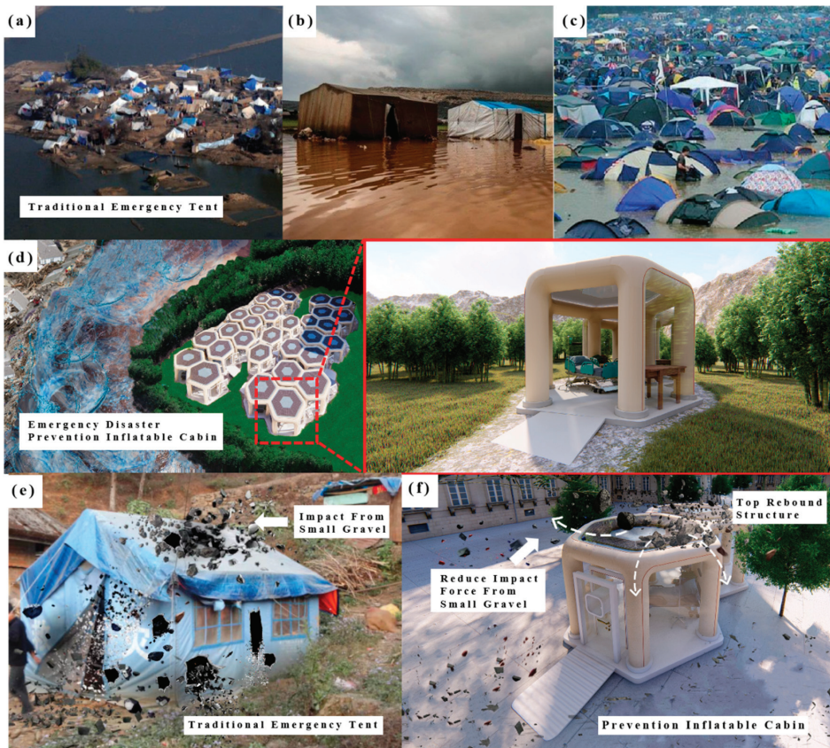
Figure 12. A comparison of traditional emergency tents and the disaster prevention inflatable cabin. (a–c) Different types of traditional emergency tents. (d) The emergency disaster prevention inflatable cabin. (e) Traditional tents face significant impact from small rubble. (f) Optimized roof elastic structure to effectively mitigate the impact of small gravel.
