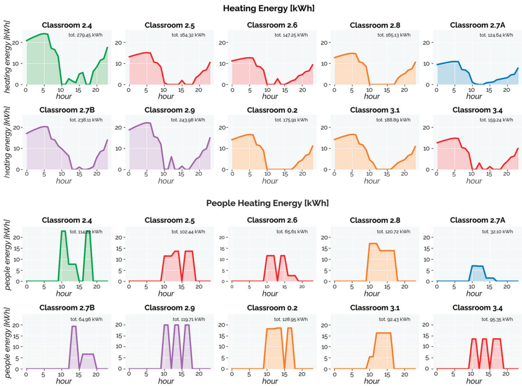
Figure 12. Visualization of hourly heating demand for some classrooms on the specified date and time. Data are colored according to the clusters identified in Figure 11.
