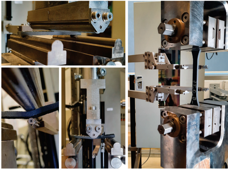
Figure 8. Experimental setup of the three-point bending test (left) and the tensile test (right) for the test specimen from fused granular fabrication and automated tape laying.
