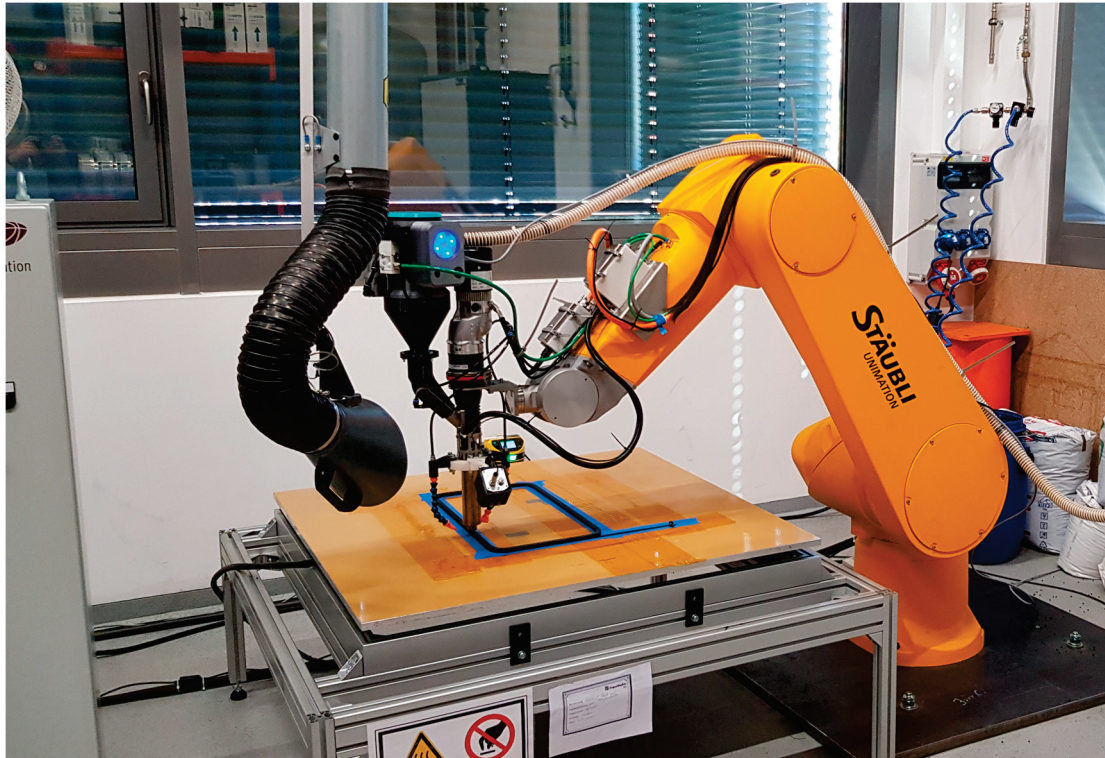
Figure 1. Fused granular fabrication unit used to produce fiber-reinforced polyamide test structures.
