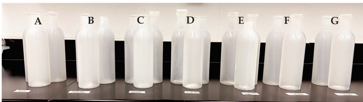
Figure 4. Various LLDPE extrusion blow-molded bottles; neat LLDPE (A) and thermally embossed LLDPE with Cu-infused \text{Mg}(\text{OH})_2 spray (B), \text{Mg}(\text{OH})_2 powder (C), \text{Mg}(\text{OH})_2 spray (D), \text{MgO} spray (E), \text{Cu}(\text{OH})_2 spray (F), and \text{ZnO} spray (G).
