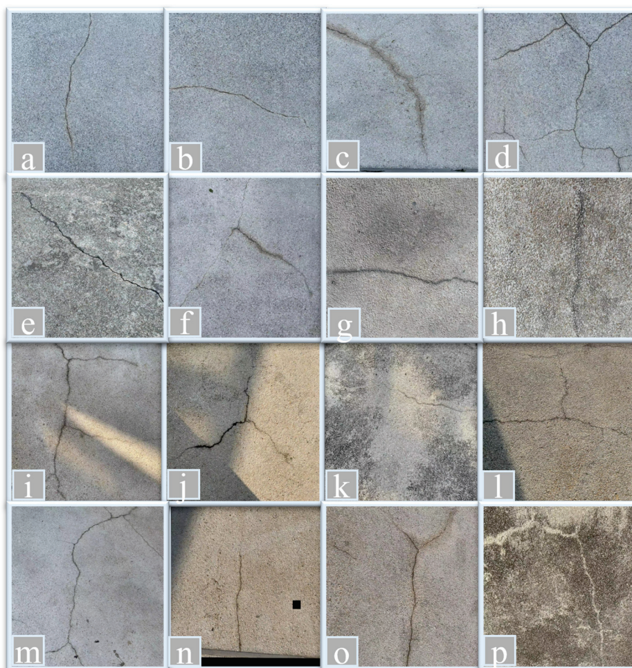
Figure 12. Sample of images from HKBCD datasets. (a–d) Different Types of cracks, (e–h) Different types of bridge materials, (i–l) Different lighting conditions and (m–p) Different types of noises.
