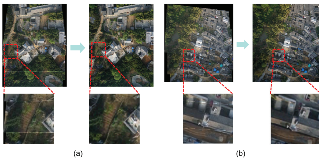
Figure 13. Comparison of seam repairment details with and without the proposed seam repairment method. (a) The first example, (b) the second example. The images with and without the proposed method for each example are placed on the left and right parts, respectively.
