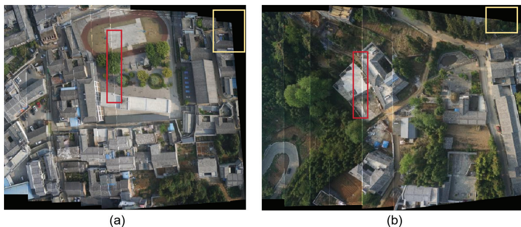
Figure 1. Irregular boundaries and stitching seams are present in the stitched images of the unmanned aerial vehicle. In the (a,b) results, the areas enclosed by the red and yellow boxes, respectively, represent portions of stitching seams and irregular boundaries.
