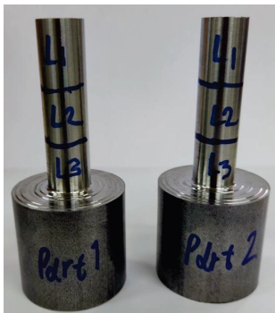
Figure 5. Machined specimens. L1, L2, and L3 denote measurement regions.
