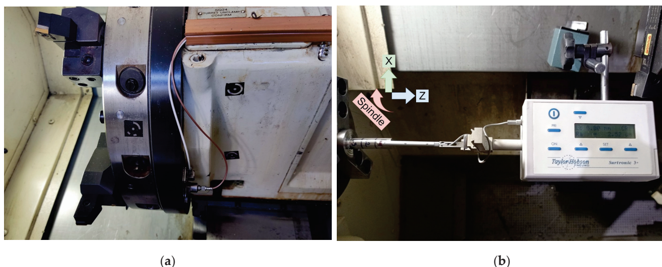
Figure 4. (a) Placement of accelerometers behind the machine tool turret; (b) Platform for measurement of surface roughness.
