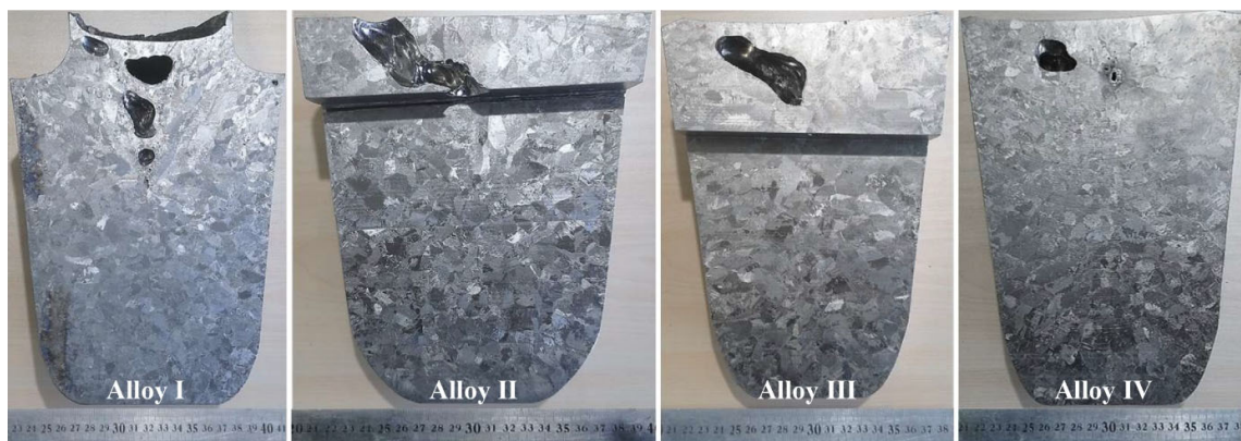
Figure 10. Macrostructure of Ti-6Al-4V alloy ingots.
