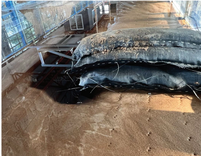
Figure 19. Localized scour pit at the head of the geotube groin following the spring tide surge.
