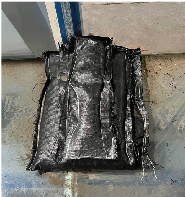
Figure 6. Geotube groin model (model dimensions: length 60 cm, width 45 cm, height 15 cm).
