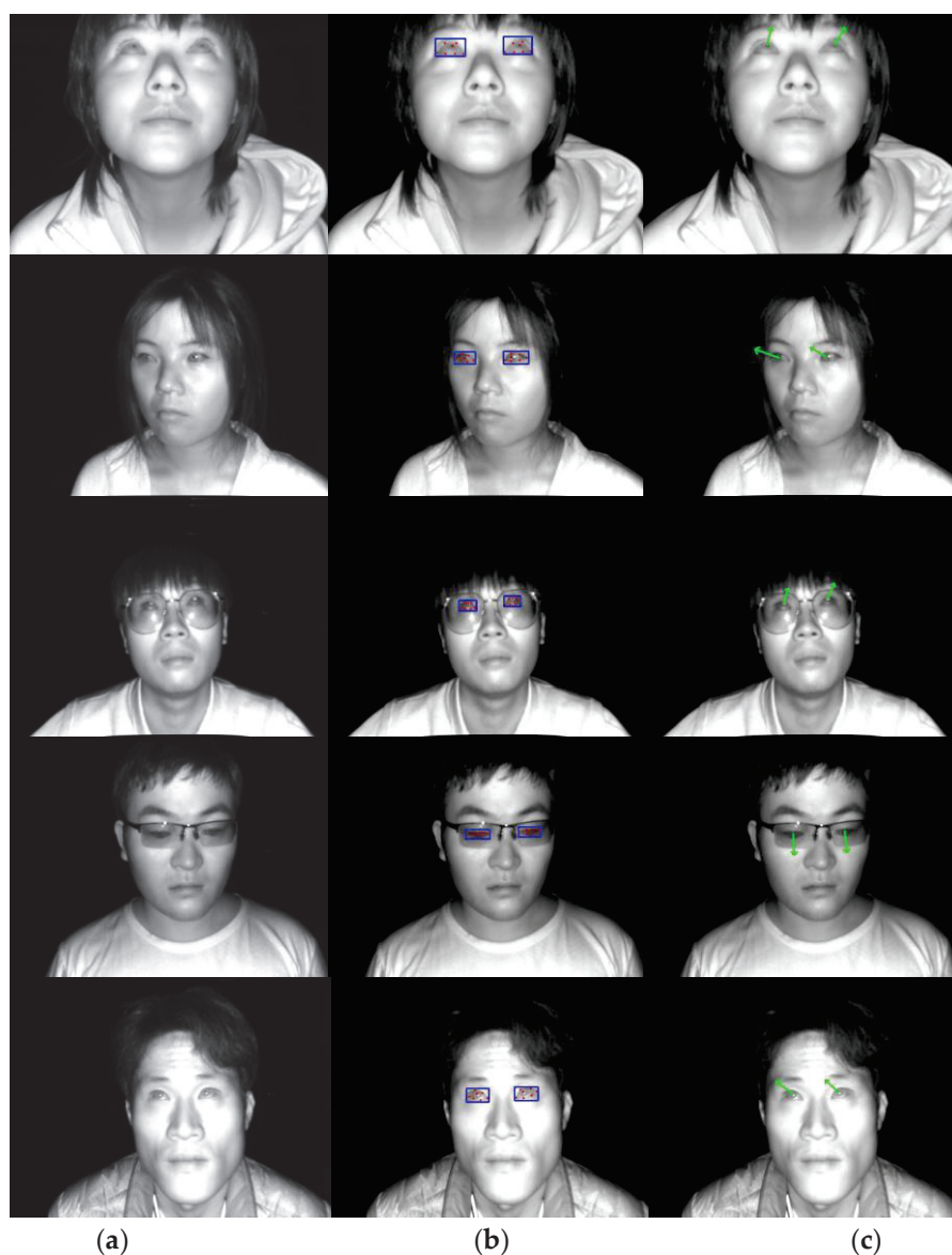
Figure 16. Results of the subject's gaze detection. Column (a) presents the original gaze images of the subject, column (b) shows the results of eye landmark detection based on YOLOv8, and column (c) visualizes the subject's gaze direction. The green arrow indicates the gaze direction detected by our model.
