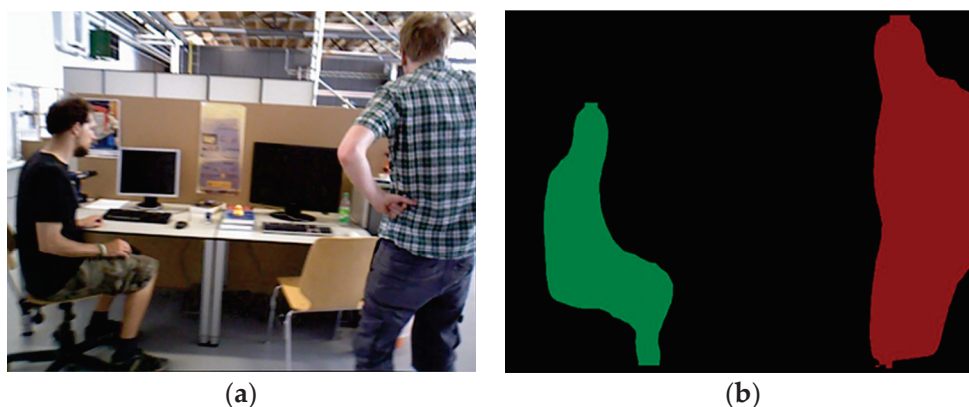
Figure 3. Dynamic object instance segmentation results. (a) Original image; (b) mask image.
