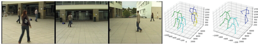
Figure 4. Estimated 3D poses and their corresponding images in an outdoor environment (Campus Dataset). Different colors represent different people detected. The penultimate column is the output result of the original voxelpose, which has misestimated the person. The last column shows the estimated 3D poses by our algorithm.
