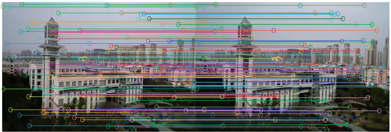
Figure 8. Schematic of feature point extraction using the SIFT algorithm.
