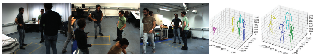
Figure 6. Estimated 3D poses and their corresponding images in an indoor social interaction environment (Shelf Dataset). The penultimate column is the output result of the original voxelpose, which has misestimated person. The last column shows the estimated 3D poses by our algorithm.
