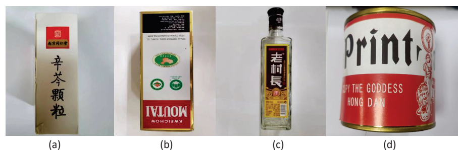
Figure 8. Actual measurement objects. (a) Smooth scene with only texture edges; (b) Scenes affected by both depth edges and texture edges; (c) Smooth surfaces affected by only texture edges; (d) Scenes with different depths of field.
