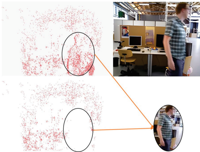
Figure 6. Comparative analysis of mapping outcomes pre and post dynamic object elimination.
