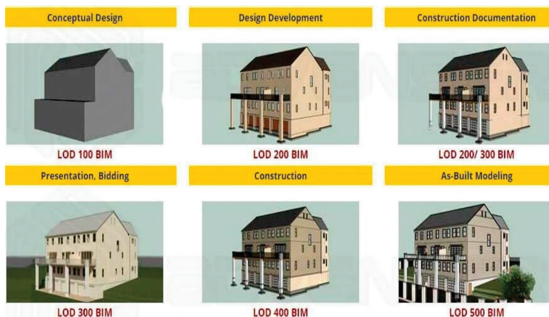
Figure 2. Relationship between the LoD and the degree of representativeness [22].
