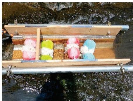
Figure 4. Zoom-in photo of the portable fishway positioned on the left side of the bank of the drainage canal.
