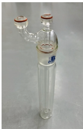
Figure 1. Schematic of glass reactor used in ozonation process.
