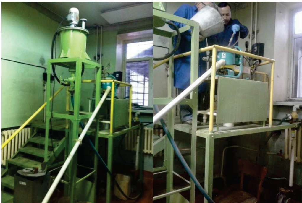
Figure 13. Knelson KS-MD 3 centrifugal concentrator and the gravitational enrichment process.
