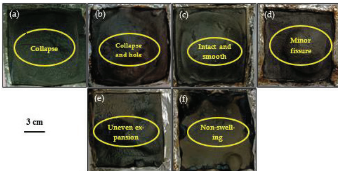
Figure 9. Residual appearance of the sample in CC including (a) B1, (b) B2, (c) B3, (d) B4, (e) B5, and (f) B6.
