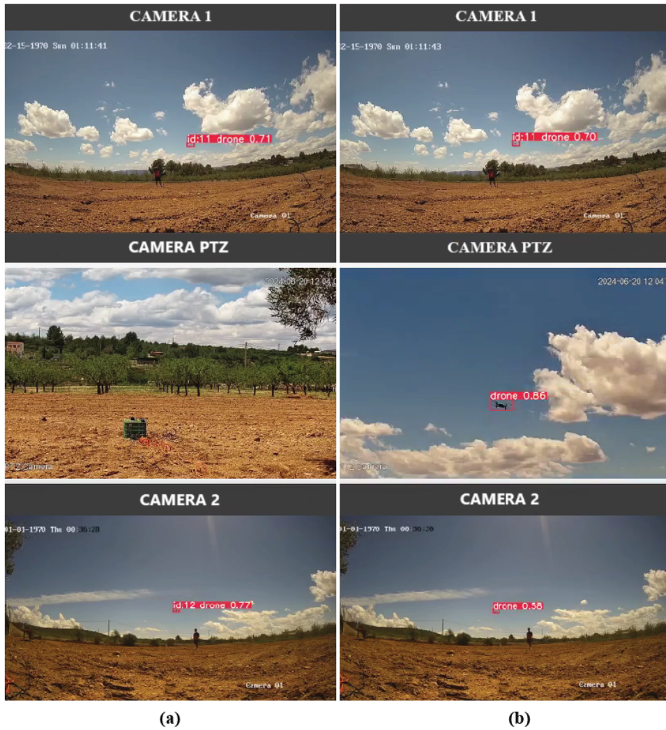
Figure 15. Vision of the cameras in the localization tests. In (a), it is shown that the fixed cameras simultaneously detected the UAV, while in (b) it is shown that the PTZ camera had already located the UAV after being provided with its exact position.
