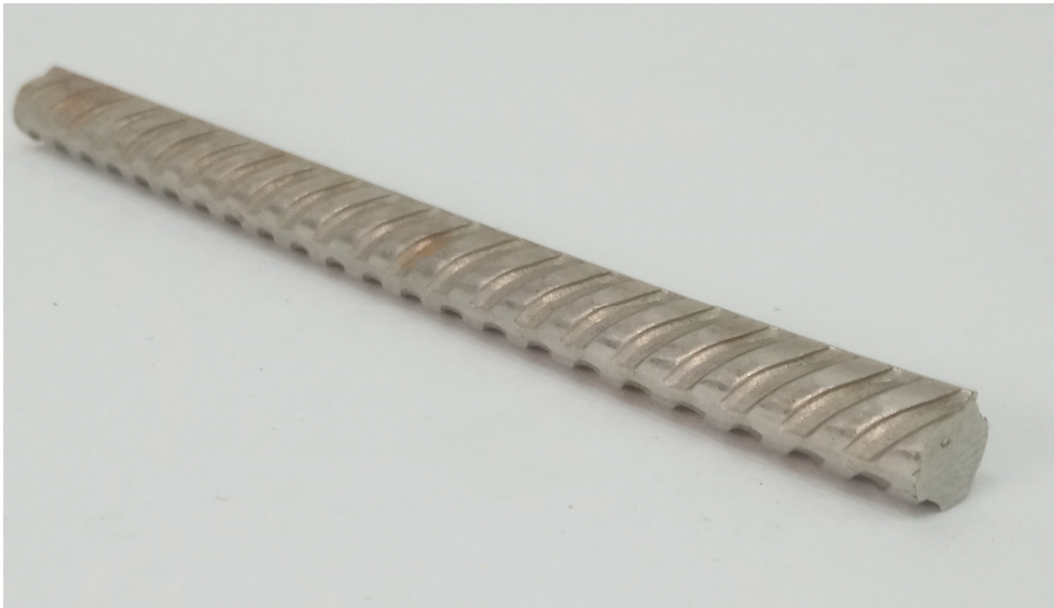
Figure 1. Standard stainless-steel rebar.
