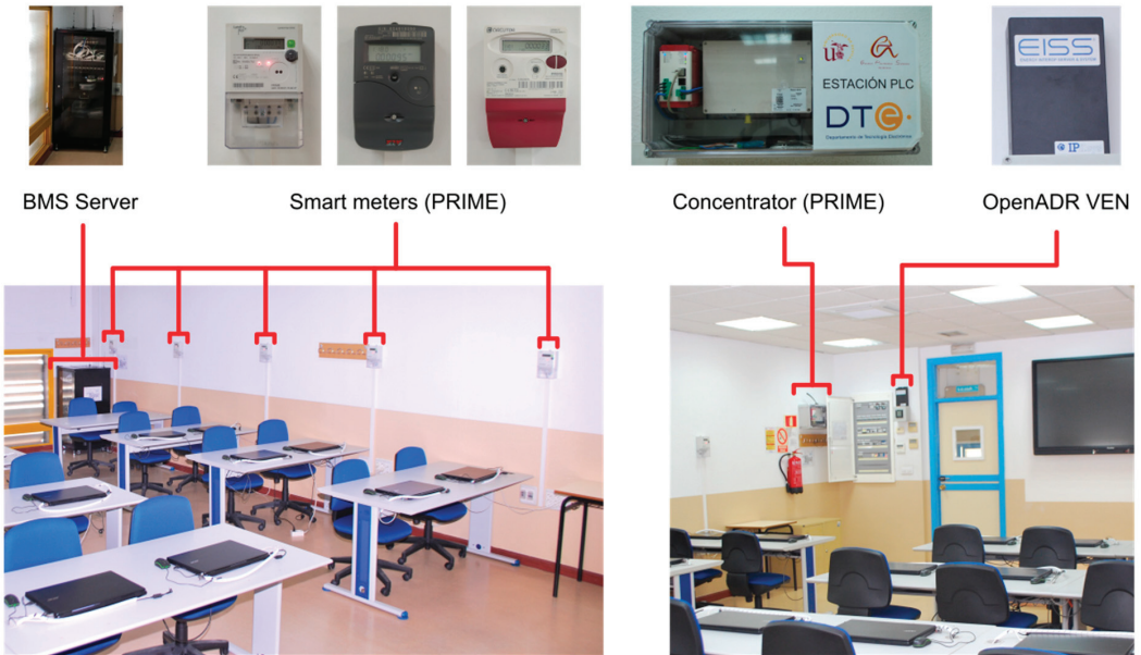
Figure 7. DERBis control and measurement devices.
