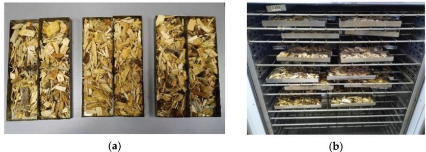
**Figure 1.** Examples of samples: (a) two sub-sample sets and (b) samples drying in the oven.
