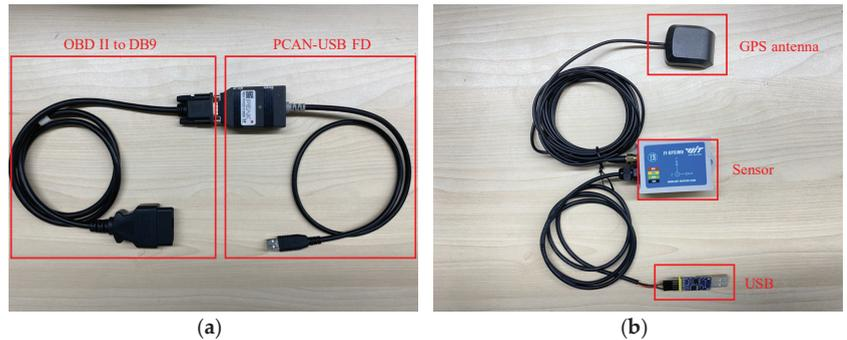
**Figure 6.** Data acquisition equipment: (a) OBD-II data collection equipment; (b) Vehicle behavior sensor.
