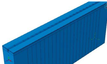
Figure 1. Numerical model of bridge–subgrade transition section.
