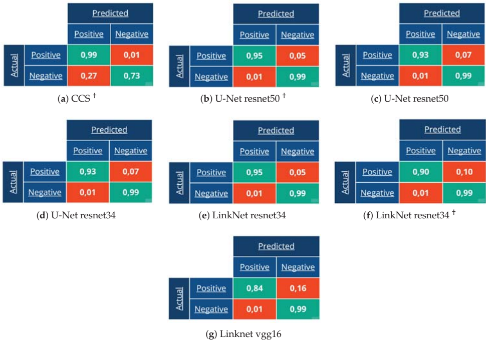
Figure 6. Confusion matrix from the prediction to (a–d) U-Net model, where (a) is CCS model, (e–g) LinkNet model. The weights of a pre-trained network with ImageNet are used to initialize each of the models (For the models † , weights were randomly initialized).
