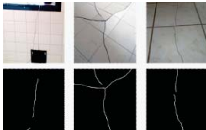
Figure 3. Examples of images collected to assemble the database and their respective ground truth (black and white).
