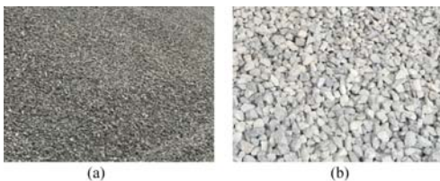
Figure 4. Two types of piles. (a) Small coarse gravel. (b) Medium coarse gravel.
