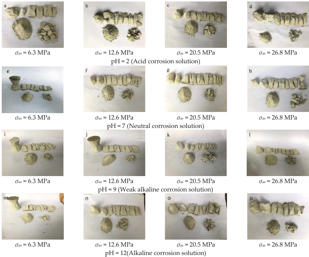
Figure 9. The destructed forms of white sandstone (a–p).
