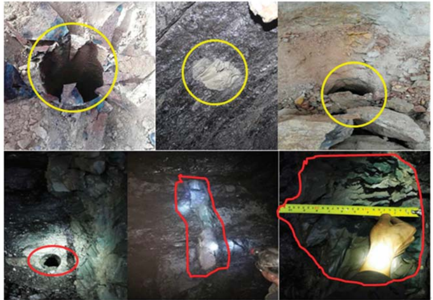
Figure 5. The positional relationship between the Ma tan 31 oil well and the coal-measure strata.
