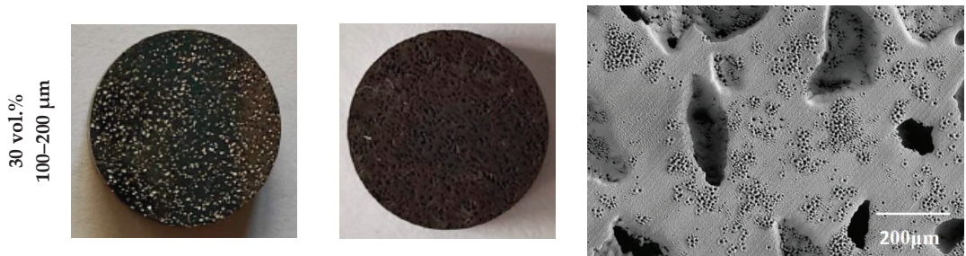
Figure 1. Optical and SEM images of some of the samples studied, before and after FS. All optical images are on the same scale, 3:1 (mm). FD: fully dense sample; 30 vol. %: sample with 30% porosity volume.
