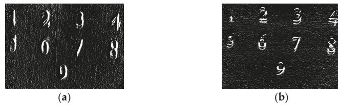
Figure 11. (a) Sobel operator on the x -axis; (b) Sobel operator on the y -axis at 100 lux.
