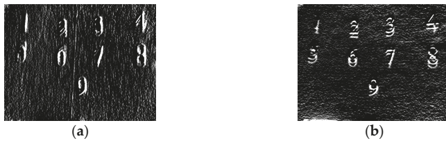
Figure 27. (a) Sobel operator on the x-axis; (b) Sobel operator on the y-axis at 2350 lux.
