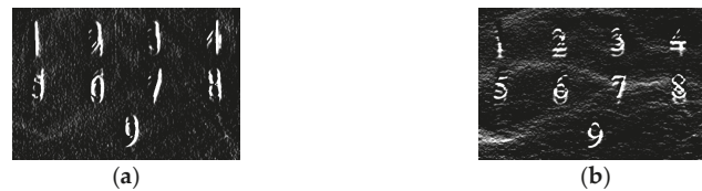
Figure 23. (a) Sobel operator on the x-axis; (b) Sobel operator on the y-axis at 2300 lux+ man shadow.
