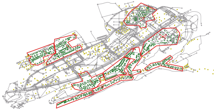
Figure 8. A map showing a solution from NSGA-II that yields the highest user coverage and the highest maximum walking distance. Covered buildings are depicted as nodes inside polygons.
