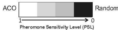
Figure 1. Symbolic illustration of the sensitive ant model showing the ants’ probability variation within the unit interval from the ACO probability when PSL = 1 to a random walk probability when PSL = 0 .
