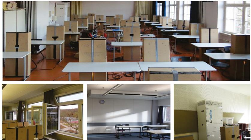
**Figure 6.** Experimental set up (top), exemplary window ventilation (bottom left), exemplary decentralised ventilation system (bottom middle), exemplary air purifier (bottom right).
