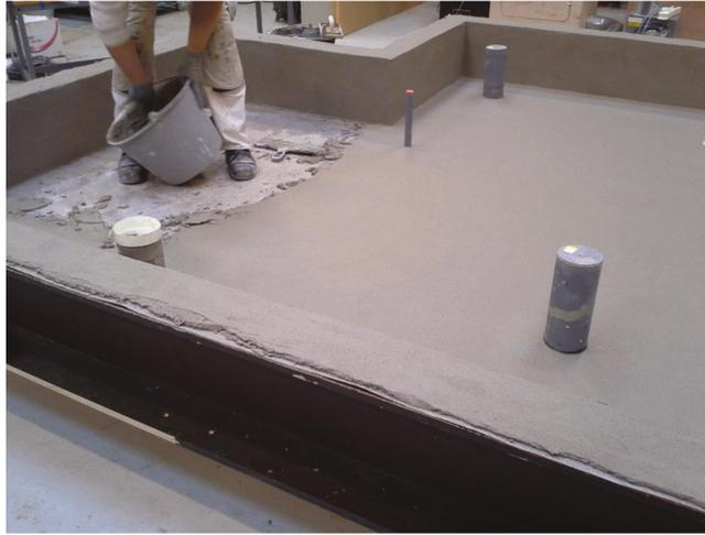
**Figure 7.** Mounting the test material inside the mock-up for System E, which is a two-component fixed mortar paste combined with edge reinforcements, epoxy and elastic pipe collars.
