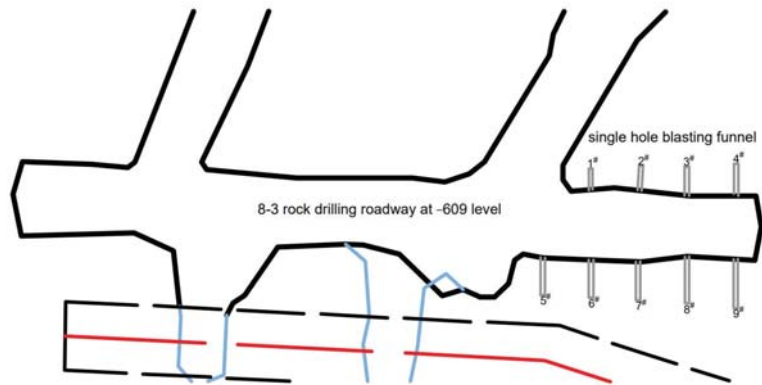
Figure 2. Schematic diagram of plane layout of blast holes in funnel test of single-hole blasting. (In the figure, # is for the convenience of numbering the holes, 1# represents hole number one, and so on).
