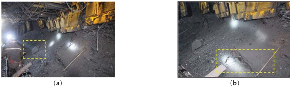
Figure 2. Failure diagram of working face. (a) Block collapse; (b) Support falling.
