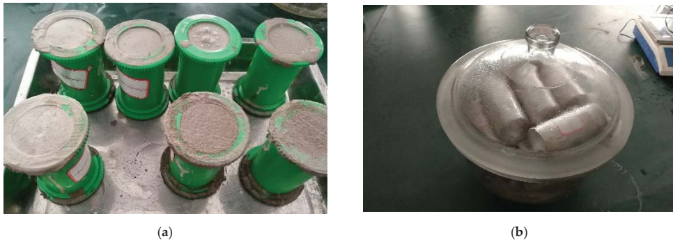
Figure 3. Preparation of MBM specimens: (a) casting MBM; (b) curing MBM.
