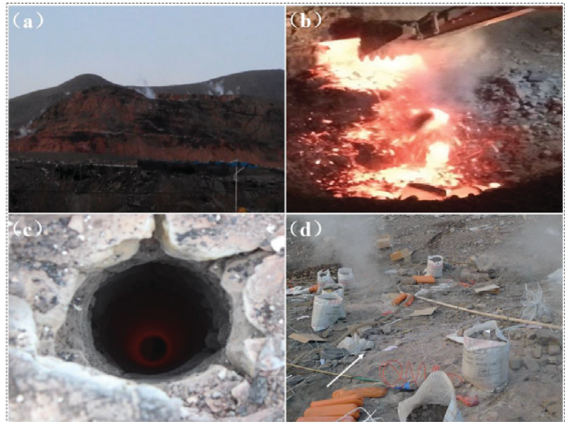
Figure 1. Blasting mining site, field photograph, December 2021, in Dashitou coalfield fires approximately 10 km northwest of Ruqigou in Ningxia province. (a) A long-time heated open pit coal mine (the color of the mountain is dark red), (b) spontaneous combustion coal seam, (c) high-temperature blast hole (the temperature can reach 400 °C) and (d) high-temperature blasting site.
