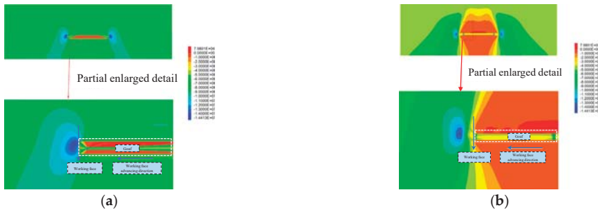
Figure 9. Local stress nephogram after grouting. (a) End section; (b) Middle section.
