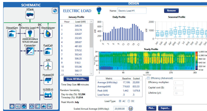
Figure 7. The proposed HRES (left) and the load demand at Basco station (right) presented in HOMER software.
