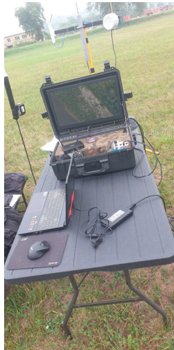
Figure 2. GCS workstation designed and built by VFD members. Photo: N. Tušnio.
