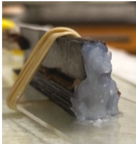
Figure 4. Salt Bridge. Capacitor in offset configuration with molded ‘salt bridge’ at one end.
