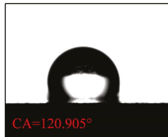
Figure 6. Wettability test of uncorroded CCC.
