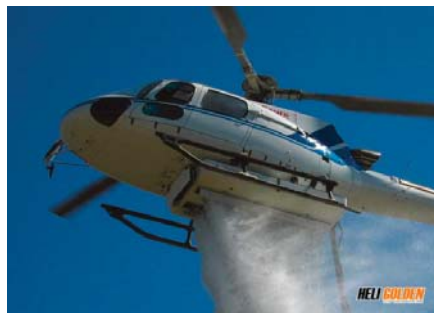
Figure 1. H125 firefighting helicopter and Isolair Eliminator II belly firefighting tank (from http://www.isolairinc.com/_gallery/4600-350A.jpg , accessed on 2 May 2022).
