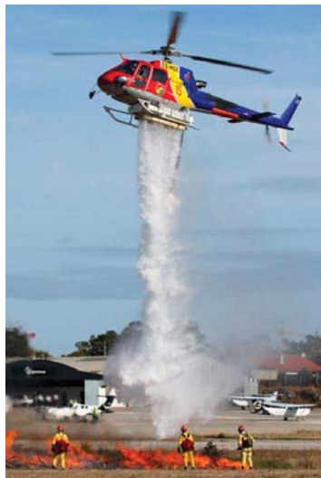
Figure 17. AS350B2 firefighting tank used for water dump firefighting (found online at http://www.isolairinc.com/_gallery/4600-350D.jpg , accessed on 2 September 2021).
