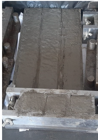
Figure 2. Poured fresh nanocalcite-doped ECC samples.
