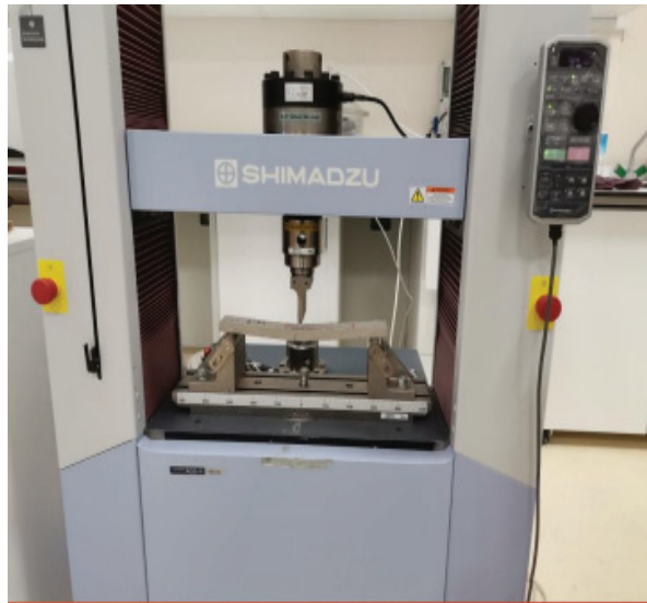
Figure 3. The flexural test set-up.
