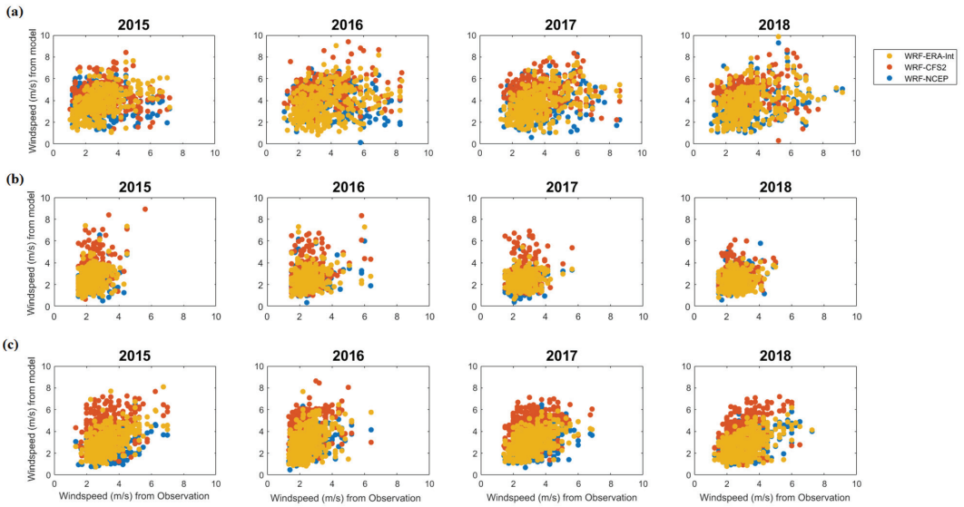
Figure A1. Daily average wind speed in \text{m s}^{-1} from the models and observations at the onshore locations (a) Shaoguan, (b) Nanping, and (c) Ganzhou.
