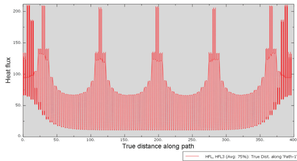
Figure 7. Heat flux ( W \cdot m^{-2} ) of each node of concrete.
