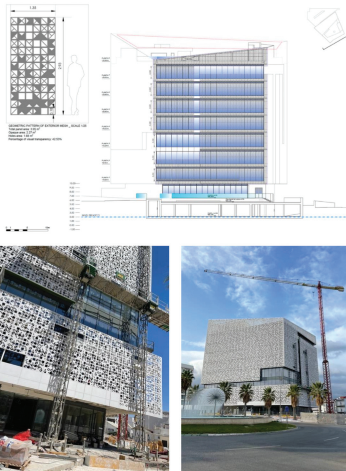
Figure 7. Double façade system with the external envelope made of lattice work. Modular geometric pattern used. South-facing elevation ( above ). Source: Castaño & Associates. LEED Rating System Report [59]. ( below ) Source: Pictures created by the author.
