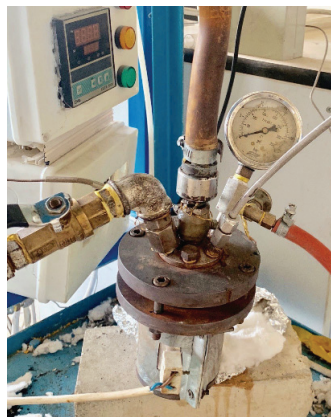
Figure 4. Photograph of the semi-batch reactor used for the thermal cracking process.
