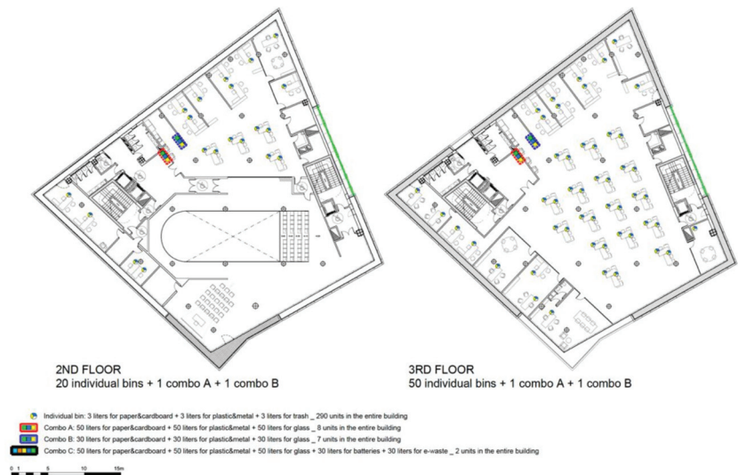
Figure 13. Location of waste collection points according to type of use and workstations. Upper floor of the Plenary Hall (first floor). Office type floor (Third Floor). Source: Castaño & Associates. LEED Rating System Report [59].
