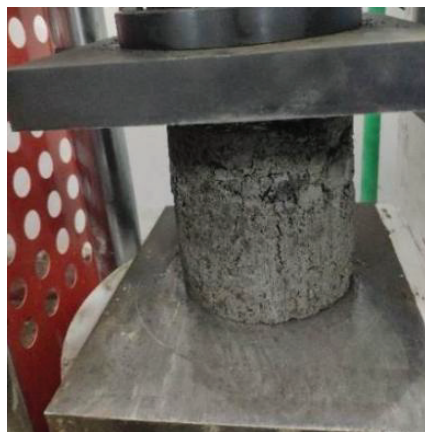
Figure 2. Axial compressive-strength test.
