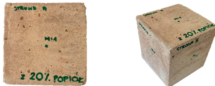
Figure 3. Ordinary concrete cube with the addition of 20% fly ash from sewage sludge.
