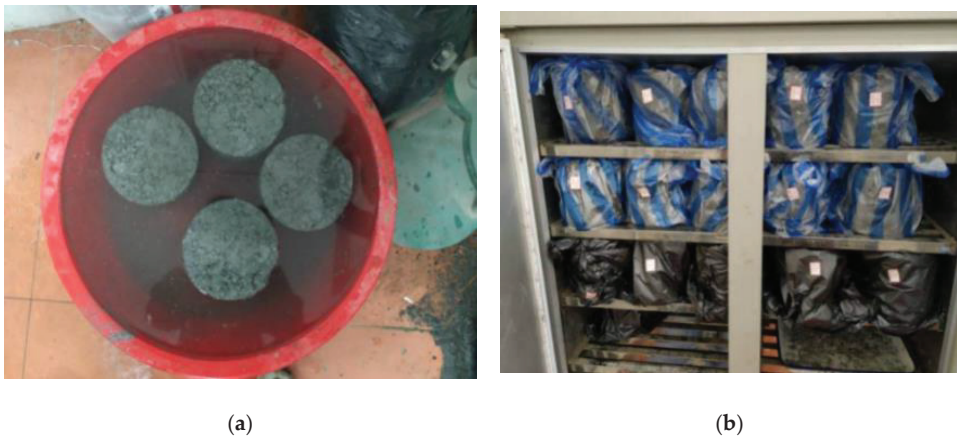
Figure 5. Shrinkage test: (a) water immersion; (b) temperature-controlled cabinet.
