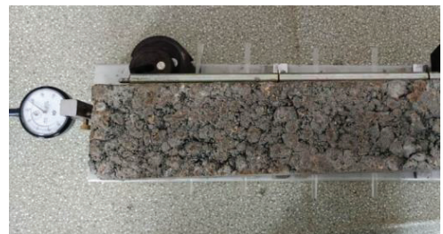
Figure 4. Compressive-resilience modulus test: (a) test setup; (b) test specimen.
