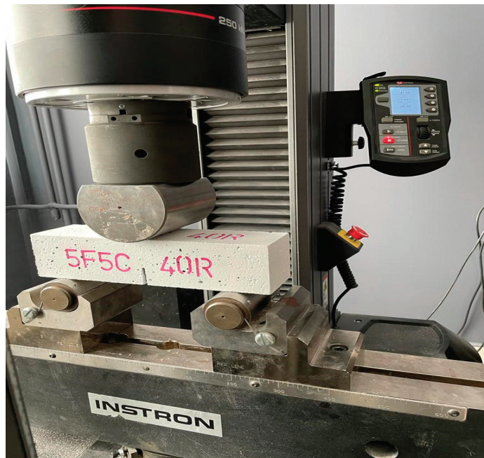
Figure 2. A notch beam under fracture energy test.
