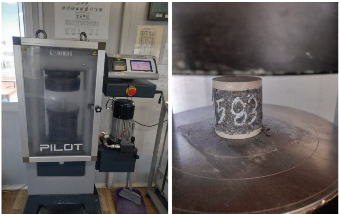
Figure 2. (a) The compressive strength test machine. (b) Cylindrical concrete specimen.
