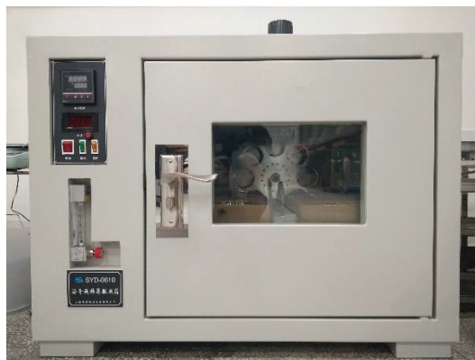
Figure 2. Rotating film oven.
