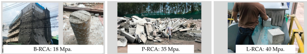
Figure 1. Recycled aggregate from various sources.
