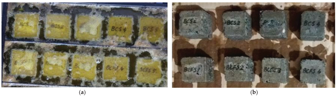
Figure 2. Resistance to the action of hydrochloric acid: (a) Specimens immersed in 18% HCl solution; (b) Specimens' aspect after 10 days of immersion in 18% HCl solution.
