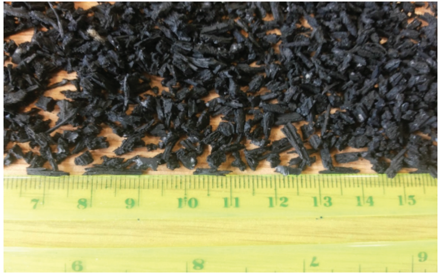
Figure 2. Crumb rubber (8 mm length) particles from worn out tyres.
