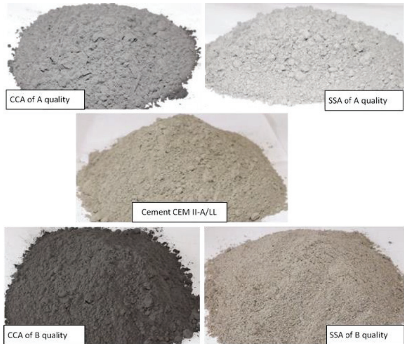
Figure 1. The SSA of A and B quality and CCA of A and B quality, compared with the cement aspect.
