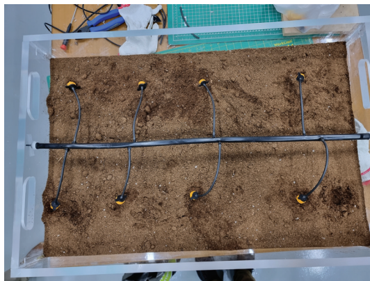
Figure 11. The addition of drip irrigation pipelines.
