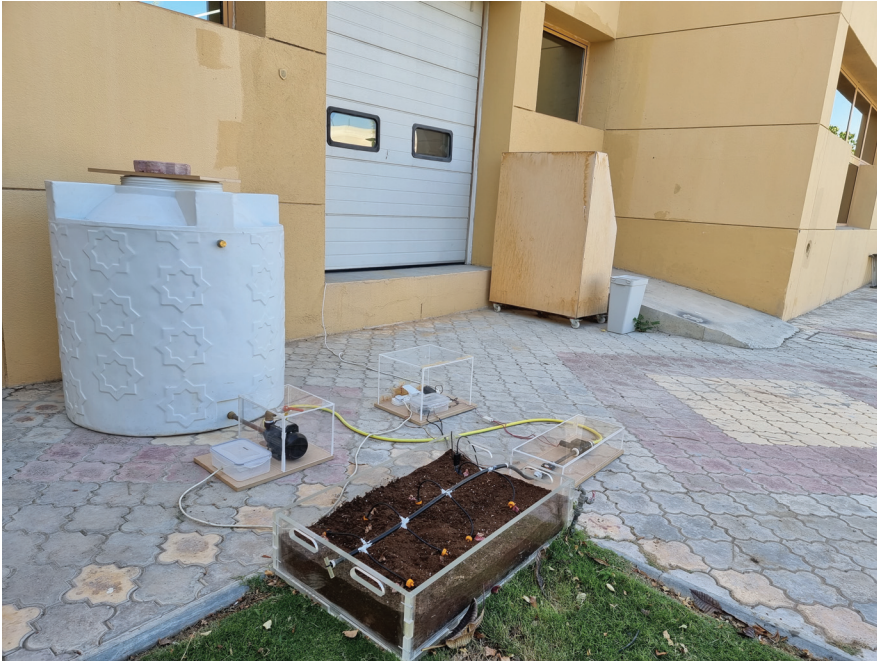
Figure 16. Smart drip irrigation system working in the field.
