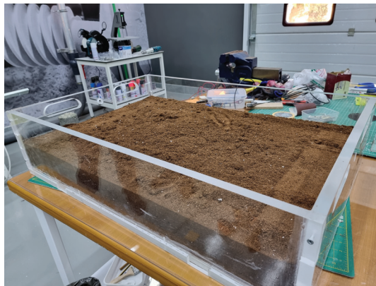
Figure 10. Adding soil to the container.
