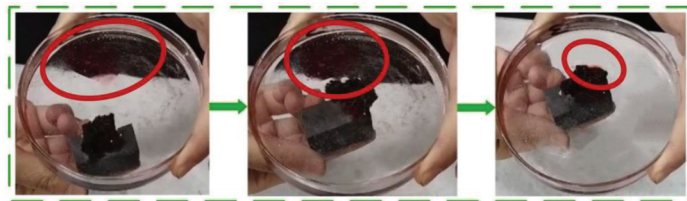
Figure 7. Oil–water separation using the MFA @ PDMS sponge.
