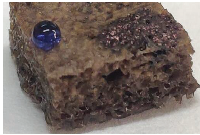
Figure 6. Hydrophobic Properties of MFA@PDMS sponge.
