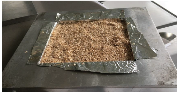
Figure 2. Stainless steel mold with ready-to-press mixture.
