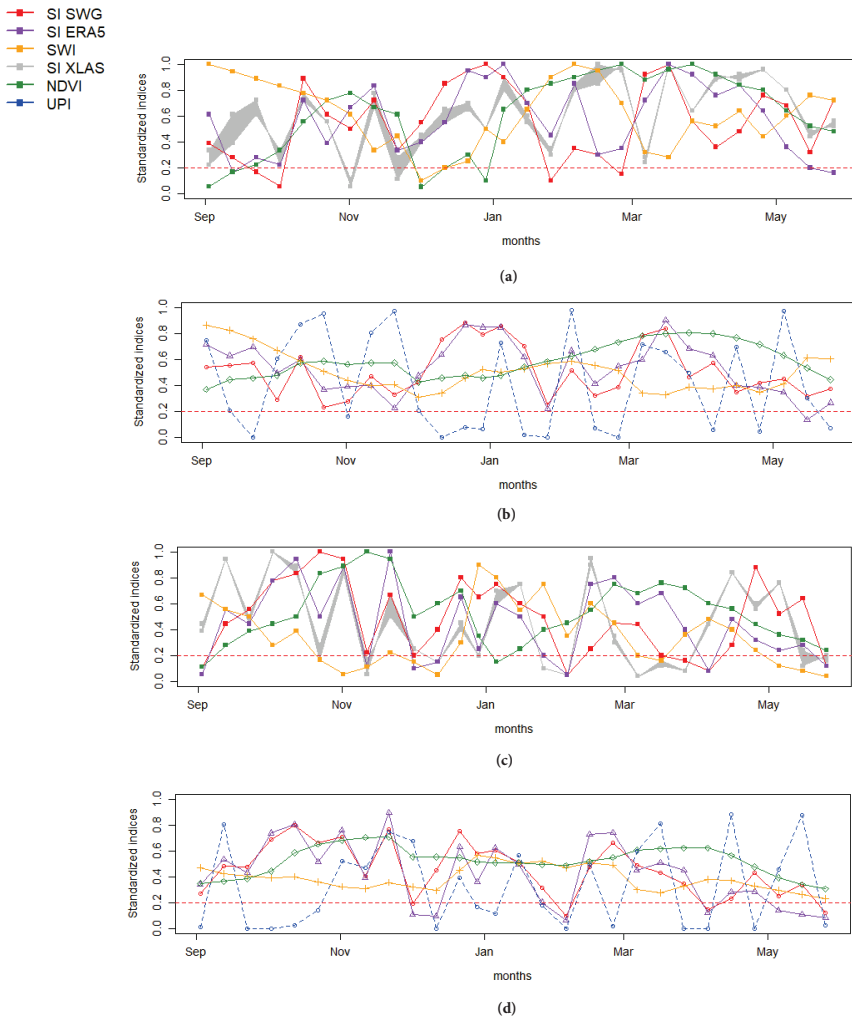
Figure 11. Decadal times series of standardized stress indices derived from different wavelenghts over the growing season of two years (2013–2014) and (2014–2015) at a local scale (a,c), in comparison with SI_{XLAS} derived from XLAS measurements over pixels containing the scintillometer transect and at a regional scale (b,d). (a) Local scale (2013–2014). (b) Regional scale (2013–2014). (c) Local scale (2014–2015). (d) Regional scale (2014–2015).
