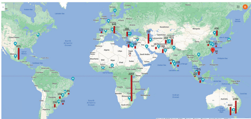
Figure 1. NTU data of carwash wastewater surveyed from Table 1.
