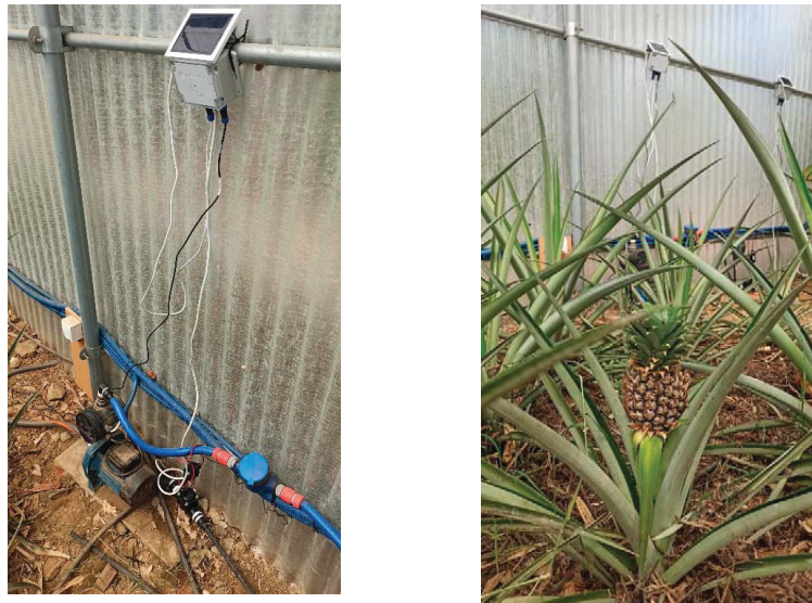
Figure 21. IoT nodes for automating the irrigation in the greenhouse.
