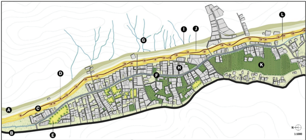
Figure 6. Proposal for the renovation of the sector of the No-Ras qanat passing through the modern village of Chavan. (A) Gentle hill way; (B) Chavan main road; (C) boardwalk; (D) No-Ras qanat's wells; (E) centre for organic farming; (F) the Jube; (G) natural seasonal streams; (H) Chavan village; (I) rainwater storage area; (J) No-Ras qanat core zone; (K) reforestation; (L) limit of the buffer zone.
