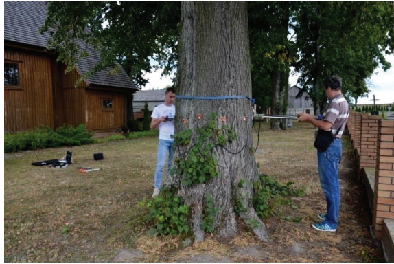
Figure 4. Measuring the geometry of the tree trunk using the PiCUS caliper (photo by M. Dudkiewicz).
