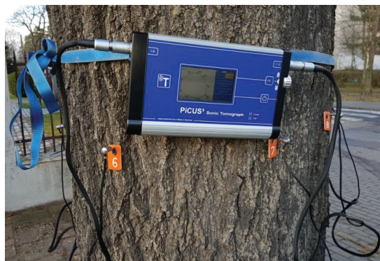
Figure 3. Acoustic tomograph CT scanner on a tree trunk (photo by M. Dudkiewicz).
