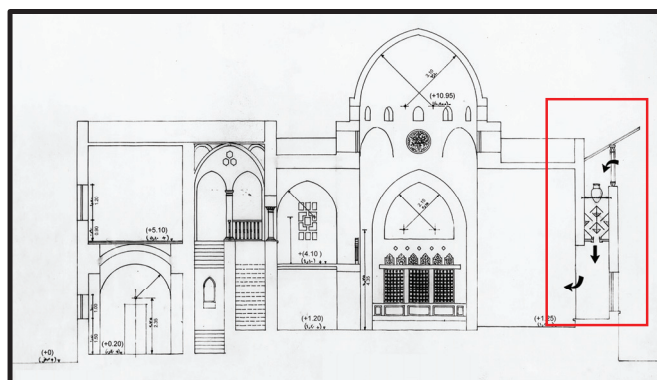
Figure 19. Section of Hamdy Seif Al-Nasr House, 1940s, the arrows signify the air flow from the wind catcher and into the space it ventilates and red boxes indicate the location of the wind catchers. Reprinted with permission from [29]. 2023. Courtesy of the Rare Books and Special Collections Library, The American University in Cairo.
