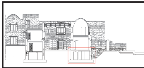
Figure 26. Villa A section showing the basement, in the red square, where the wind from the windcatcher is directed and cooled down.
