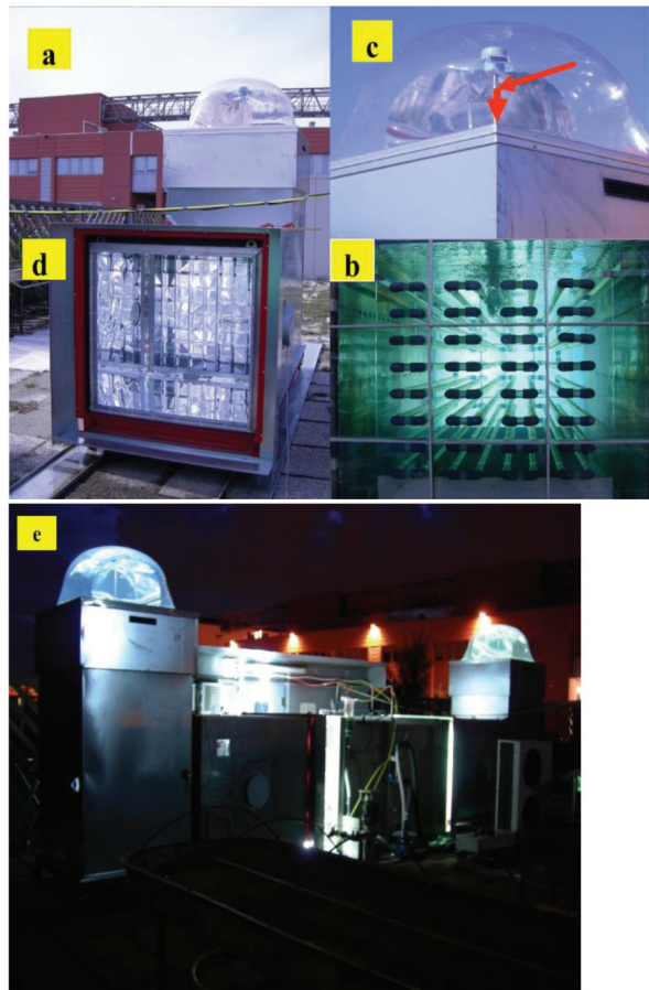
Figure 8. The 110 L photobioreactor utilized for the hydrogen production experiments. (a) General view of the photobioreactor; (b) frontal view of the photobioreactor; (c) sun-tracking mirrors collecting light; (d) light ducts delivering light to the photobioreactor from the opposite sides; (e) nocturnal view of the photobioreactor with two light bulbs (1000 W each) placed in the light duct to provide illumination to the culture during the night.
