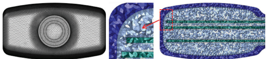
Figure 2. Generation mesh in the computational domain.
