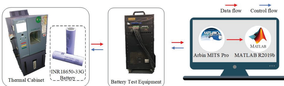
Figure 2. Outline of the test bench: offline calibration and schedule condition application.
