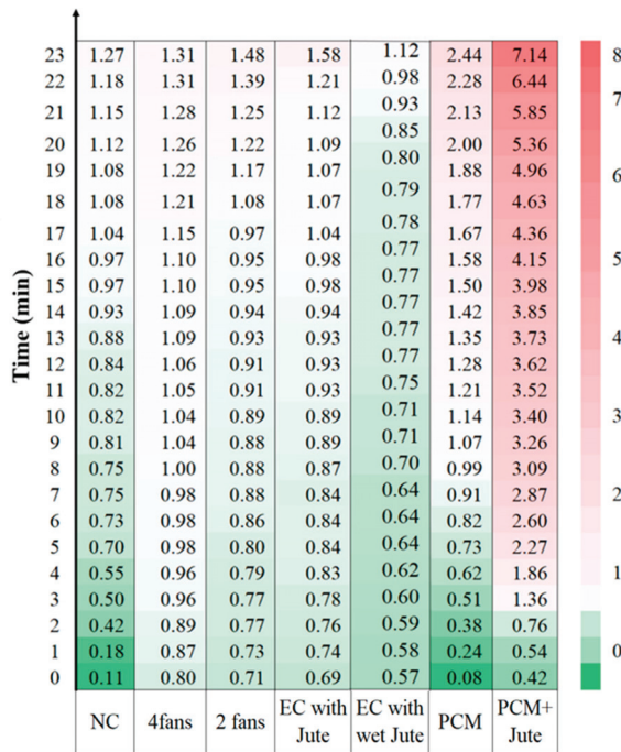
Figure 12. Comparison of nonuniformity temperature distributions for all the discussed cooling strategies.
