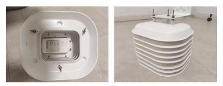
Figure 5. Outdoor temperature and relative humidity sensors (with solar radiation shield).
