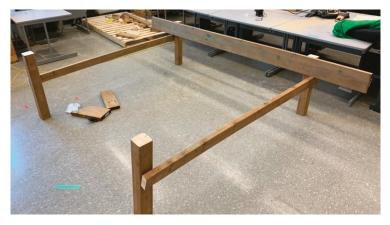
**Figure 2.** The 2  $\times$  8 beam installed between the back posts, with temporary 2  $\times$  4 lateral bracing installed between the left and right posts.
