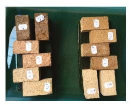
Figure 5. Specimens cut and accommodated over the saturated Oasis.
