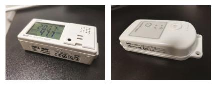
Figure 4. Temperature and relative humidity sensors for indoor (left) and outdoor (right) environments.
