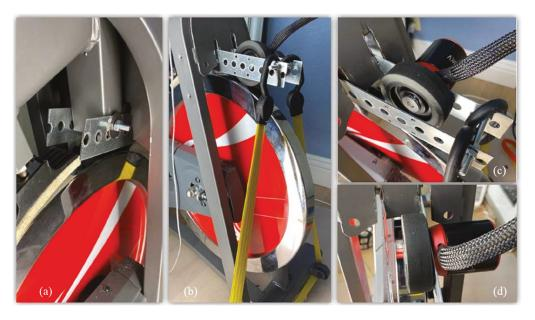
Figure 8. The motor assembly in the prototype (a) the modification of the bike frame to mount the motor; (b) the friction drive assembly; (c) the friction drive and the motor assembly; and (d) a closer view of the friction drive with the Motor.
