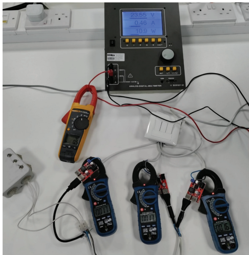
Figure 9. Experimental set-up of load sharing between parallel buck cells.
