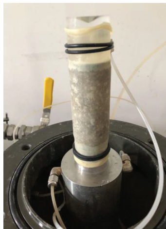
Figure 3. Specimen for triaxial compression test.
