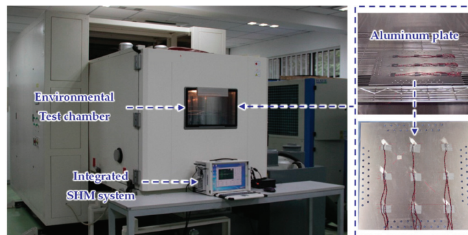
Figure 8. Experimental system of temperature influence on LW.
