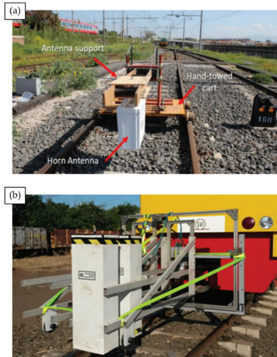
Figure 4. A selection of leading GPR systems. (a) Ballast fouling inspection trolley with selectable-frequency GPR antenna module [77]. (b) Loco-mounted fixed directional air-coupled GPR antennas.
