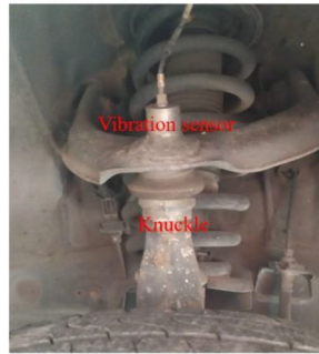
Figure 2. The vibration sensor.
