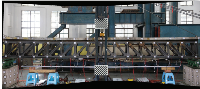
Figure 18. Test beam image after perspective transformation process.
