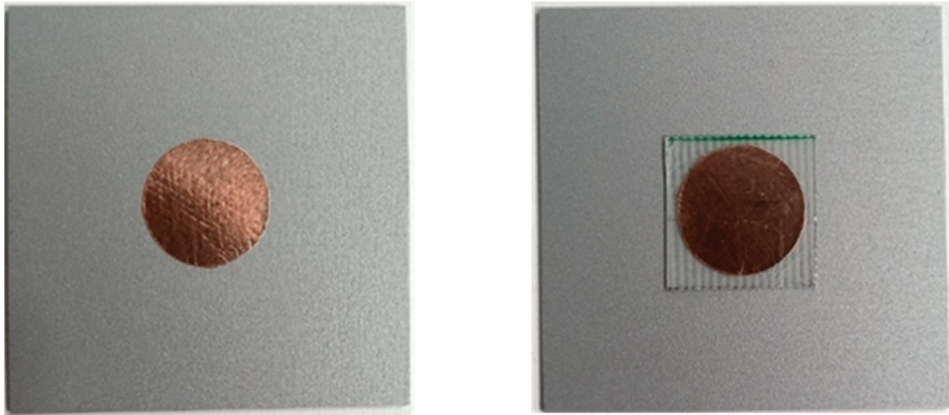
Figure 7. The manufactured Chipless RFID Tag deployed onto the same without (left) and with (right) the substrate layer.
