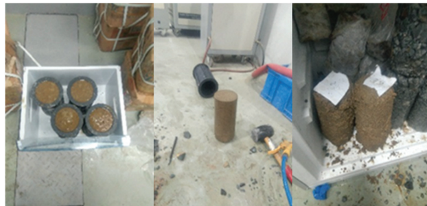
Figure 1. Preparation of sand specimen.
