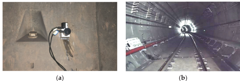
Figure 21. Field test diagram. (a) Acceleration measuring point of tunnel wall. (b) Overall view.
