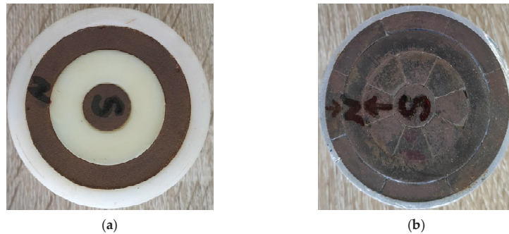
Figure 14. The fabrication of permanent magnets of (a) the ring-type EMAT and (b) the flux-concentrating EMAT.
