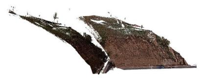
Figure 19. Initial point cloud of landslide in two phases.
