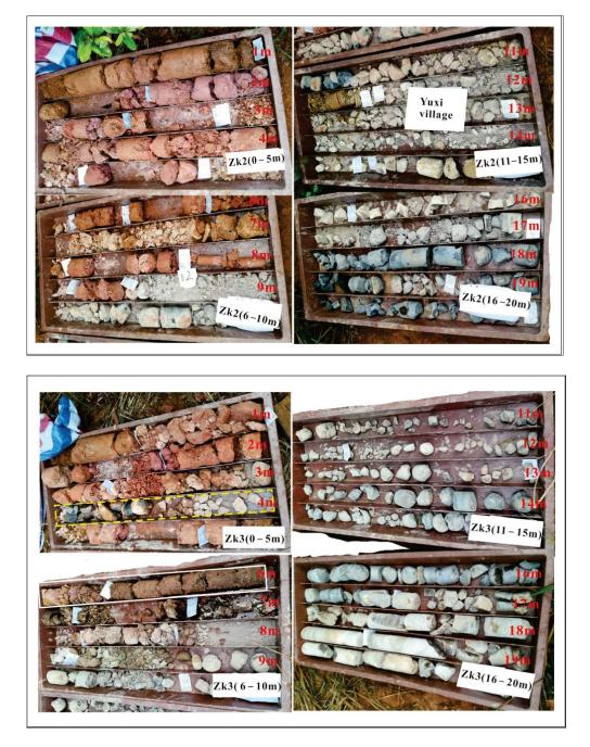
Figure 4. Drilling core samples from three boreholes (ZK1, ZK2, ZK3).
