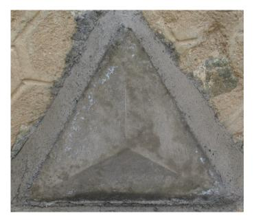
Figure 8. Triangular pyramid target.
