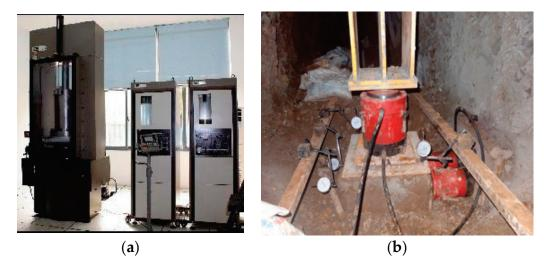
**Figure 3.** Laboratory and in situ tests. (a) Model MTS815–03 Triaxle Tester. (b) Original rock shear test.
