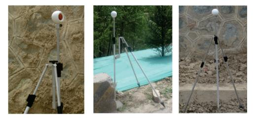
Figure 10. Prism ball target.
