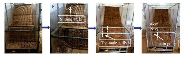
**Figure 8.** Scour failure process during three rounds of rainfall: (a) First round of the first rainfall event lasted for 5 min, (b) First round of the first rainfall event lasted for 70 min, (c) First round of the second rainfall event lasted for 120 min, (d) Third round of the third rainfall event lasted for 120 min.
