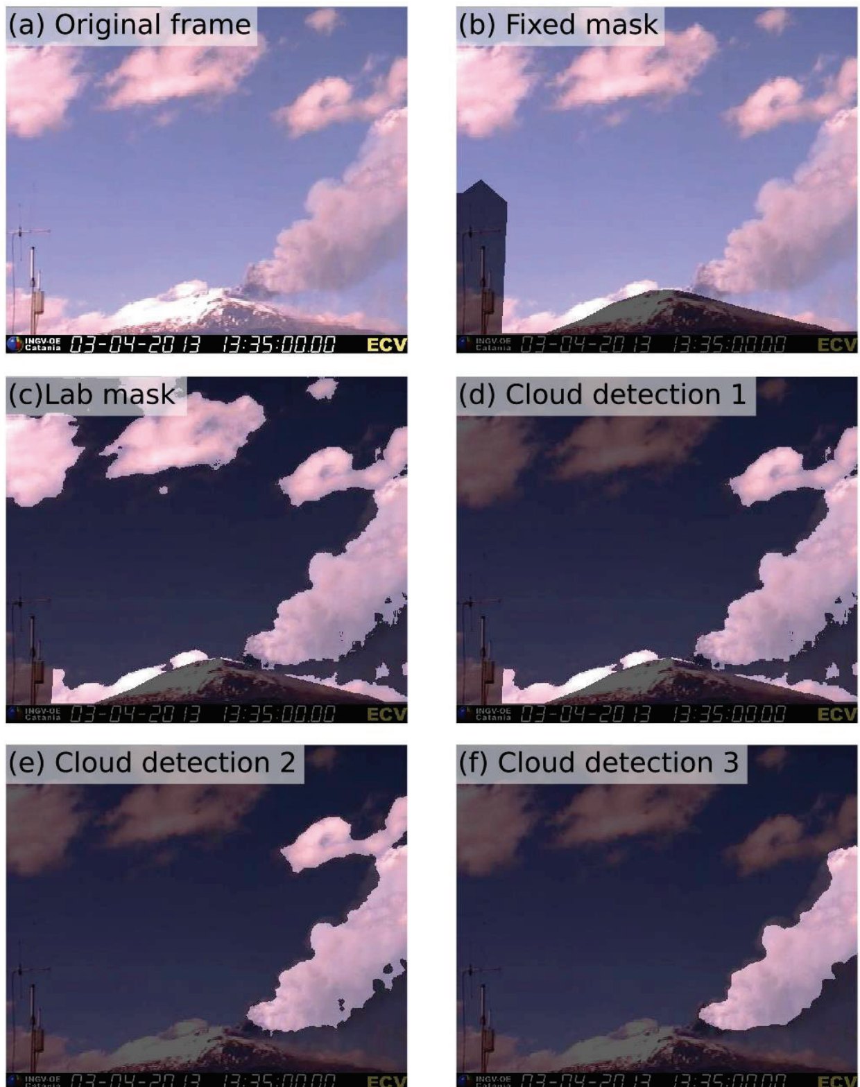
Figure 1. Illustrative example of the application of the procedures used to identify the plume in the program PHA. (a) Original image. (b) Application of the fixed mask. (c) Application of the Lab mask. (d–f) Application of the different algorithms aimed at discarding the clouds from the image.
