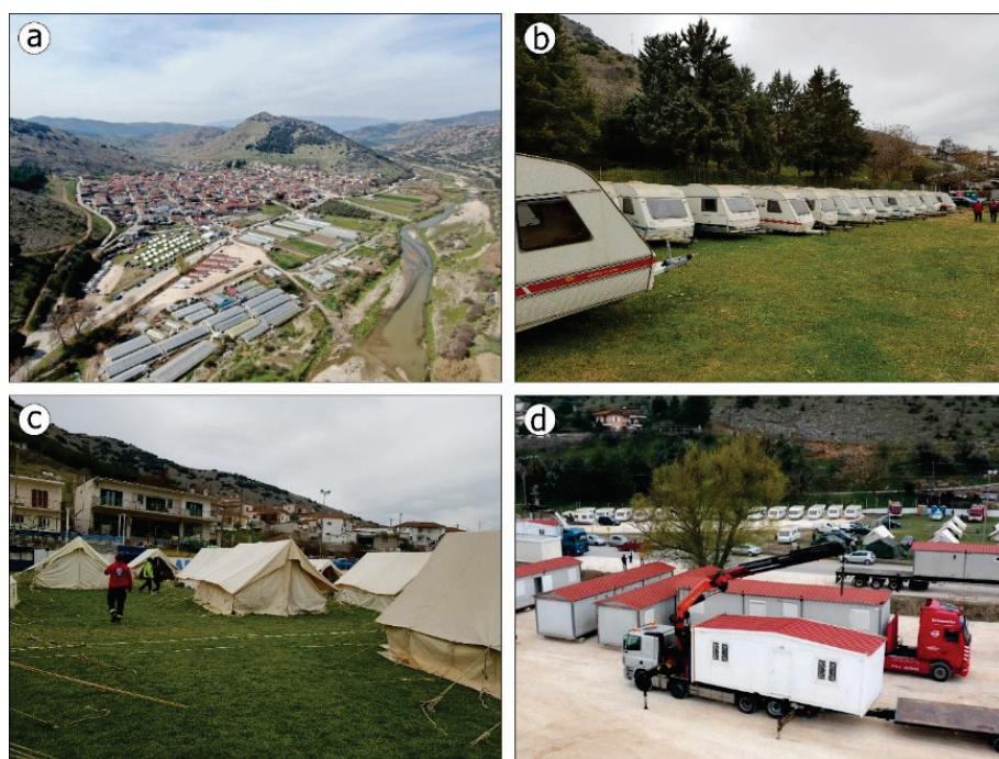
Figure 4. Several types of emergency shelters for the immediate housing of people in need after an earthquake which were used at the Damassi (Thessaly) camp (a) after the 3 March 2021 Thessaly earthquake. They comprised (b) camper vans, (c) tents, and (d) temporary container-type structures in the same area. Amid the pandemic, the use of many different types of shelters contributed to the avoidance of overcrowding in camps and the maintenance of physical distance in order to limit the spread of the novel virus in the earthquake-affected community.
