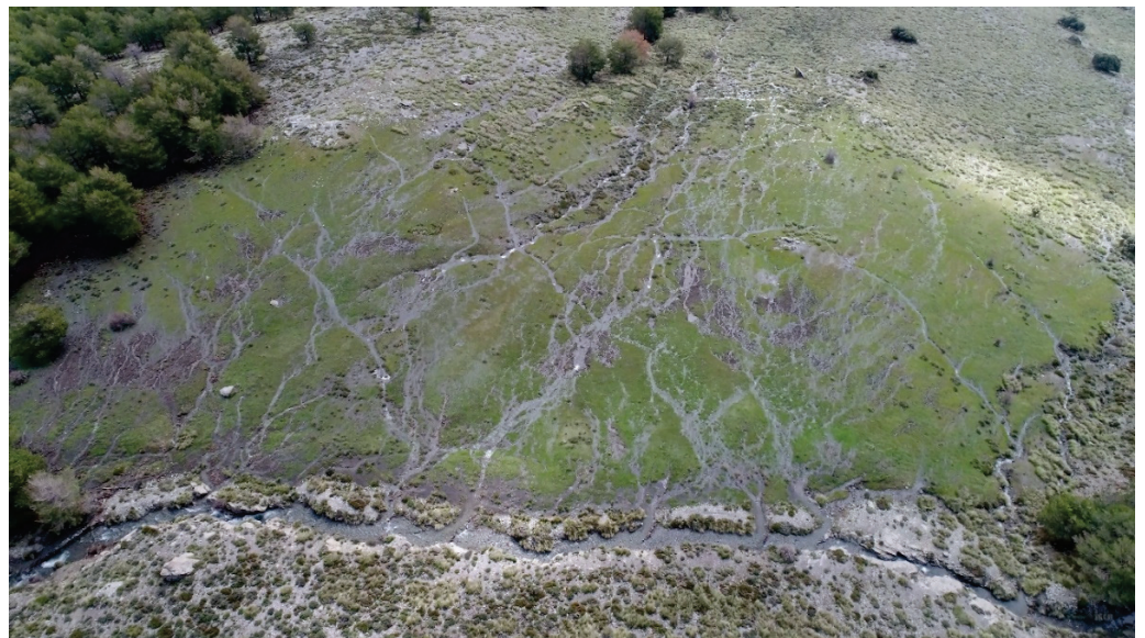
Figure 2. Example of an area where water flowing through a careo channel is released for infiltration. The infiltration zone is 6 km from the beginning of the channel. When the photograph was taken (April 2021), a flow rate of 250 L/s infiltrated. The seepage water generates pastures in the neighboring infiltration zones. (Photo: Blas Ramos).
